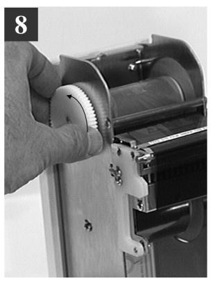
Fasten the end of the dye film onto the Take-up Core with a small piece of adhesive tape, and wind on a couple of turns. Avoid creasing of the dye film and position it centrally on the core.
